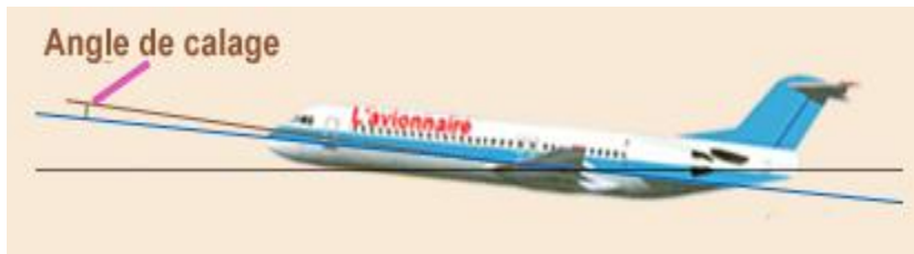
Figure II.16 : Angle de calage
