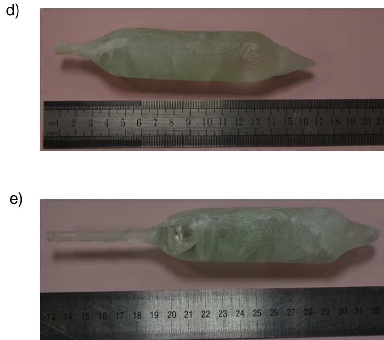
Figure 3.9 : Cristaux sans recuit : a) LGT2, b) LGT3, c) LGT4, d) LGT6 et e) LGT7
