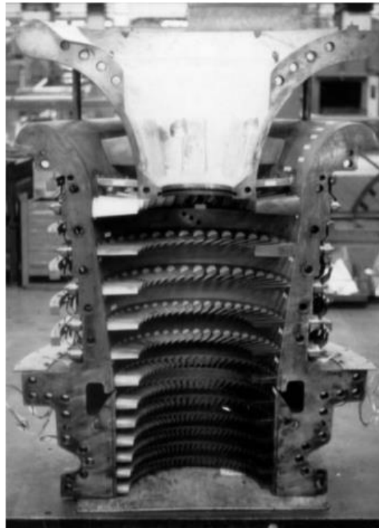
Fig.17 shows an example of stator blades fitted on the PGT10 turbine inlet casing.
